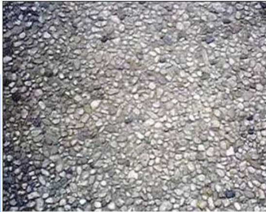
Exposed Aggregate Finish Using Nafuclar W
